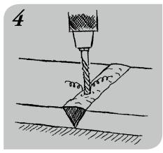
After appr. 30 min. the seam will behardened and can be machined mechanically. It is possible to grind, to spatule or to drill. To adapt the seam formed to the appearance of the original material apply laquer.
