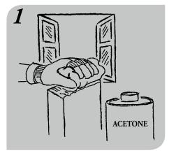
The faces of the parts to be connected must be cleaned thoroughly from dirt, grease, oil and adhesive agent residuals. To be recommended for the cleaning: acetone. During these workings the room must be ventilated well.
